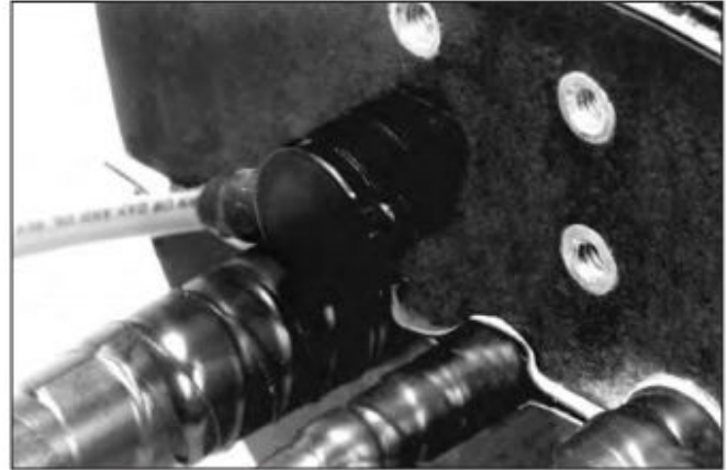
External Isolation Terminal
