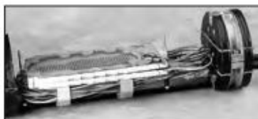
Buffer Tube Management System for a 6.5" x 22" (165 x 559 mm) COYOTE Splice Case
